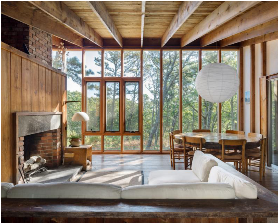
Walling's Halprin House, Wellfleet (1965). The living room window wall was achieved using only 2-by-4's and strips of plate glass.
